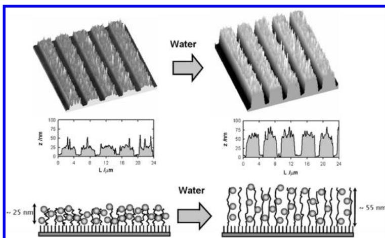
**Figure 4.22** Patterned IL-based polyelectrolytes brushes loaded with AuNPs, in compressed and swollen states (left and right, respectively). Top, middle: AFM images and cross-sectional analyses of patterned brush layers, obtained in air and water; bottom: schematic corresponding to AFM data [70]. Reproduced by permission of The Royal Society of Chemistry.
