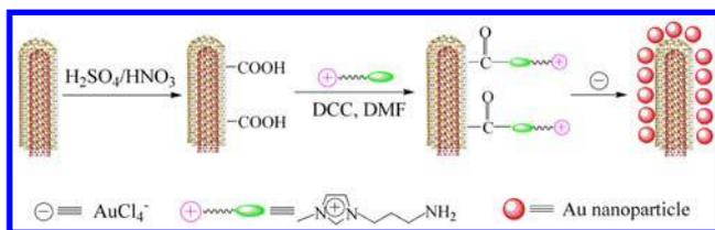
**Figure 4.17** Illustration of the preparation procedures of CNT-IL-Au Reprinted from Carbon, 46, Wang, Z., Zhang, Q., Kuehner, D., Xu, X., Ivaska, A., and Niu, L., The synthesis of ionic-liquid-functionalized multiwalled carbon nanotubes decorated with highly dispersed Au nanoparticles and their use in oxygen reduction by electrocatalysis, 1687–1692, copyright 2008, with permission from Elsevier.
