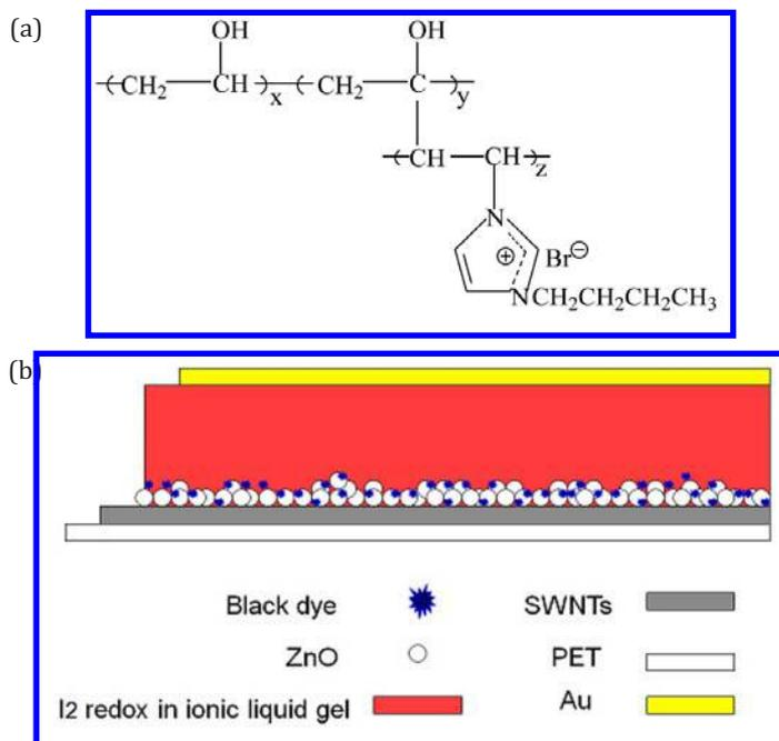
**Figure 4.13** Structure of (a) PVA-g-VIC4Br and (b) solid-state DSSC. Reproduced with permission from Wei, D., Unalan, H. E., Han, D. X., Zhang, Q. X., Niu, L., Amaratunga, G., and Ryhanen, T. (2008). A solid-state dye-sensitized solar cell based on a novel ionic liquid gel and ZnO nanoparticles on a flexible polymer substrate. *Nanotechnology*, **19**, pp. 424006–424010.
