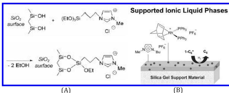
**Figure 4.3** Immobilization of chloroaluminate-based ionic liquid by grafting of imidazolium chloride (A) and the scheme of the concept of supported ILs (B). From Mehnert, C. P. (2005). Supported ionic liquid catalysis. *Chem. Eur. J.*, **11**, pp. 50–56. Copyright Wiley-VCH Verlag GmbH & Co. KGaA. Reproduced with permission.
