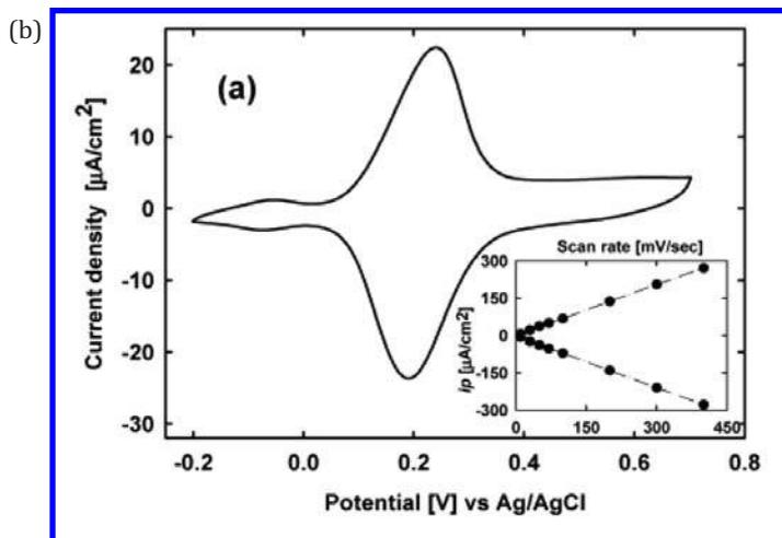
**Figure 4.6** (a) Schematic representation of IL-based polyelectrolytes brushes. (b) Cyclic voltammogram corresponding to electroactive brush (14 nm).  $v$ : 30 mV/s. Supporting electrolyte: 5 mM KCl. Inset: Plot of anodic and cathodic peak currents versus  $v$ . Reprinted with permission from Ref. [47]. Copyright 2007 American Chemical Society.
