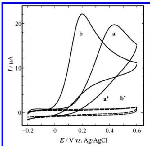
**Figure 4.7** CVs for the oxidation of AA (1.0 mM) at bare (curve a) and 1-butyl-3-methyl imidazolium chloride ([BMIM][Cl])-modified (curve b) GC electrodes in 0.10 M phosphate buffer. Curves a and b represent CVs obtained at the above electrodes in the same solution containing no AA. Scan rate, 100 mV s<sup>-1</sup>. Reprinted with permission from Ref. [48]. Copyright 2005 American Chemical Society.
