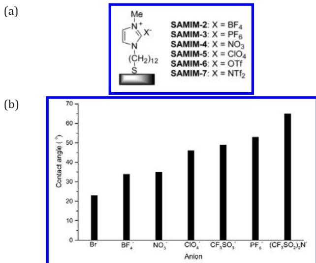
**Figure 4.5** Self-assembled monolayers presenting imidazolium ions at the tail ends on Au having different anions (a) and the effects of counteranions on surface hydrophilicity and hydrophobicity (b). Reprinted with permission from Ref. [46]. Copyright 2004 American Chemical Society.
