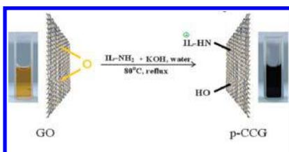
**Figure 4.20** Illustration of the preparation of polydisperse chemically converted graphene (p-CCG) from graphite oxide (GO) by amine-terminated IL [67]. Reproduced by permission of The Royal Society of Chemistry.
