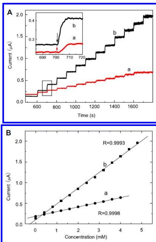
**Figure 4.11** (A) Steady-state response of (a) GOD/sol-gel/GC and (b) GOD/PFIL/sol-gel/GC electrodes with successive addition of glucose concentration (0.4 mmol/L each step). Applied potential: 1.05 V vs. Ag|AgCl (in saturated KCl). Inset shows a magnification of the second addition of glucose. (B) Calibration curves of the above (a), (b) electrodes. Reproduced with permission from Ref. [52]. Copyright Elsevier (2007).
