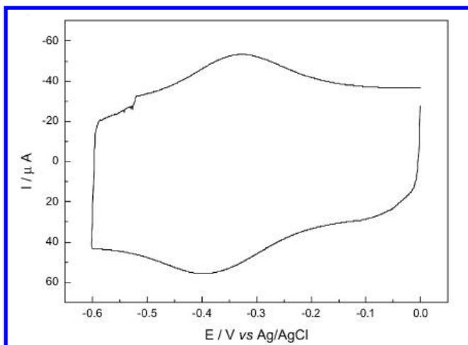
**Figure 4.8** Cyclic voltammogram at the HRP/CNTs/1-butyl-3-methylimidazolium hexafluorophosphate-modified glassy carbon electrode in 0.1 M phosphate buffer solution (pH = 7.00) under nitrogen. The scan rate is 0.1 V/s. Reprinted with permission from Ref. [49]. Copyright 2004 American Chemical Society.
