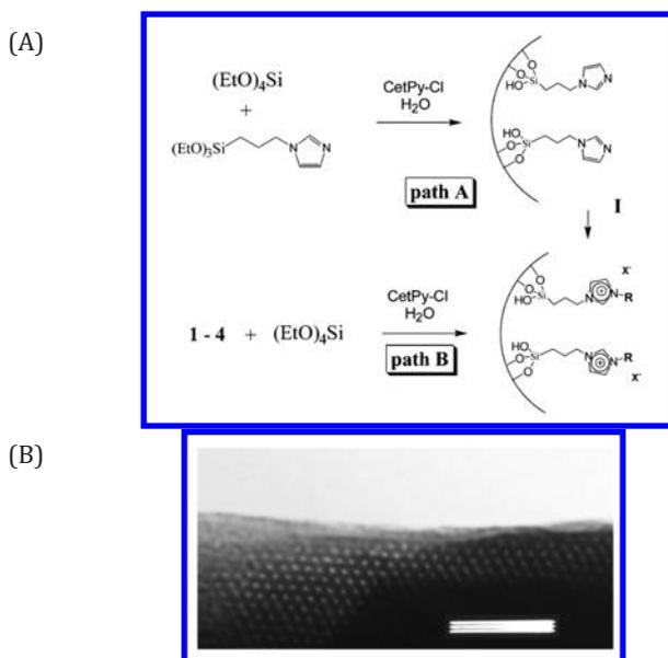
**Figure 4.4** Schematic (A) and TEM image (B) of Immobilization of ionic species on the surface of mesoporous nanostructured silicas [45]. Reproduced by permission of The Royal Society of Chemistry.
