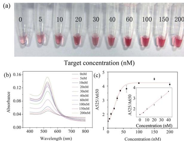
**Fig. 9** (a) Photographs of AuNP aggregates after incubation with different concentrations of target DNA followed by digestion by exonuclease III, (b) corresponding UV-vis spectra, and (c) the standard curve for the relationship between the ratio of 525 nm over 650 nm and the concentration of target DNA, the inset: linear relationship between the ratio of  $A_{525}/A_{650}$  and the concentration of target DNA.
