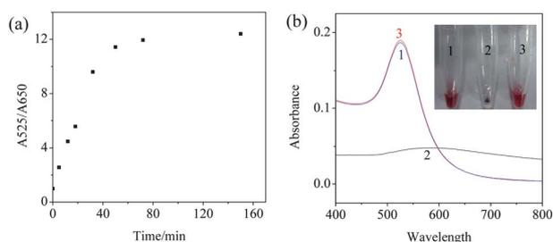
**Fig. 5** (a) Time course study of disassembly of AuNPs (with a 12-nucleotide gap) monitored by the ratio of 525 nm over 650 nm. (b) Absorption spectra of dispersed DNA-AuNPs (1), AuNP aggregates (2), and redispersed AuNPs in solution after incubation for 50 min in the presence of oligomer  $F_d$  (3). The insert shows corresponding photographs.
