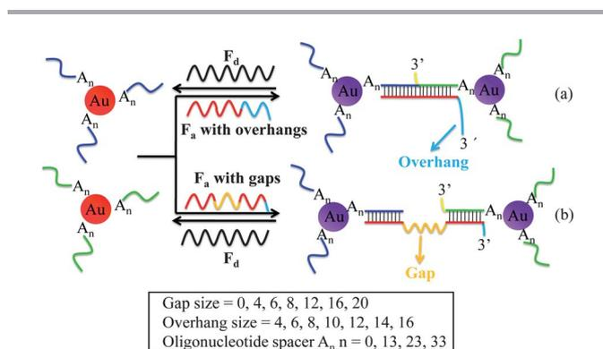
**Fig. 1** Scheme of DNA-directed assembly and disassembly of DNA-functionalized AuNPs. Oligomer  $F_a$  contains overhangs (a) and gaps (b).
