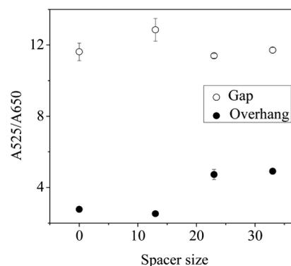
**Fig. 4** The disassembly rate of AuNPs monitored by the absorption ratio of 525 nm over 650 nm as a function of spacer size in the presence of oligomer  $F_a$  containing a 12-gap nucleotide (open circles), and that in the presence of oligomer  $F_a$  containing a 12-overhang nucleotide (solid circles).
