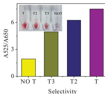
**Fig. 10** Histogram of specificity of the DNA assay. No T: no target DNA was added, T: perfectly matched DNA was added; T2: two-base mismatched DNA; T3: three-base mismatched DNA. The DNA concentrations of T, T2 and T3 are 40 nM. [Linker DNA] = 100 nM. [Exonuclease III] = 60 U. Inset: the photograph of the corresponding samples. All DNA sequences are listed in the ESI.†
