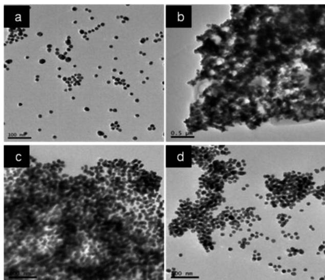
**Fig. 8** TEM images of (a) mono-dispersed colloidal AuNPs, (b and c) AuNP aggregates after adding exonuclease III, and (d) AuNP aggregates after digestion by adding the target and exonuclease III. Scale bars in (a), (c) and (d) are 100 nm, and that in (b) is 500 nm. [Target] = 60 nM, [exonuclease III] = 60 U.
