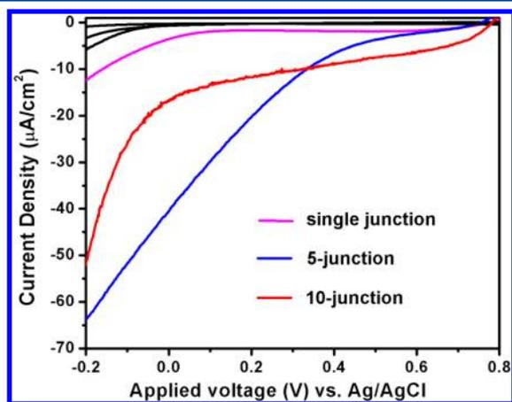
**Figure 7.**  $J-V$  curves of three photoelectrodes (single-junction photoelectrode, 5-junction photoelectrode, and 10-junction photoelectrode) with the same total thickness but different single-layer thicknesses.
