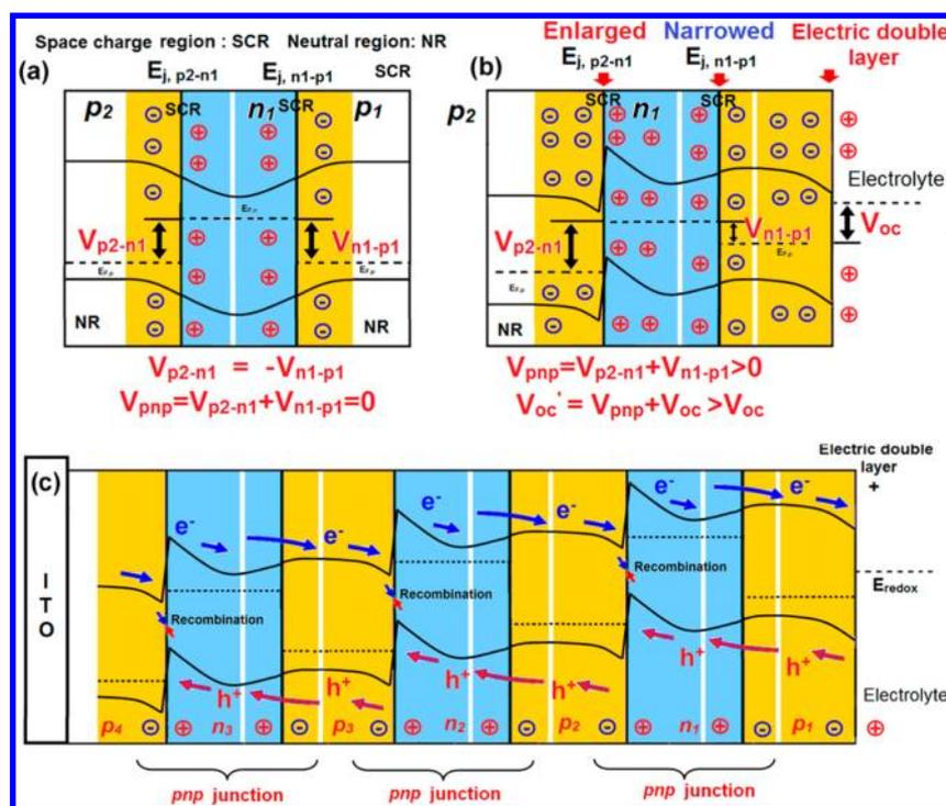
**Figure 8.** (a) Schematic of a single  $pnp$  junction under light irradiation. (b) Schematic of a  $pnp$  junction electrode in the electrolyte under light irradiation. (c) Schematic of a multilayer  $pnp$  junction electrode in the electrolyte under light irradiation.
