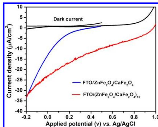
**Figure 2.** Current density vs potential ( $J$ - $V$ ) curves of the 15-junction photoelectrode (red line) and single  $\text{CaFe}_2\text{O}_4/\text{ZnFe}_2\text{O}_4$  photoelectrode with the same thickness (blue line).
