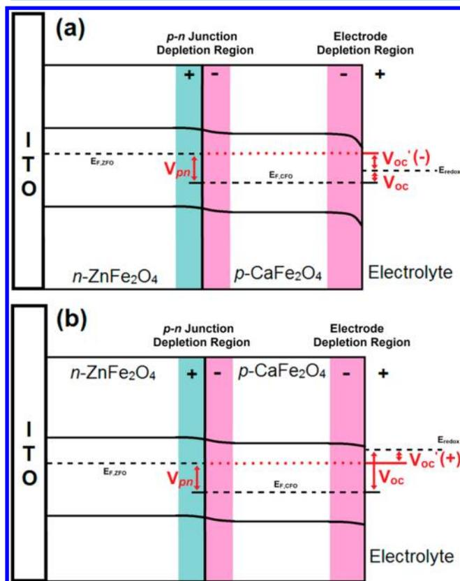
**Figure 5.** (a) Band structure of CaFe<sub>2</sub>O<sub>4</sub>/ZnFe<sub>2</sub>O<sub>4</sub> junction at the sudden of the light irradiation. (b) Band structure of CaFe<sub>2</sub>O<sub>4</sub>/ZnFe<sub>2</sub>O<sub>4</sub> junction under the light irradiation after getting stable.
