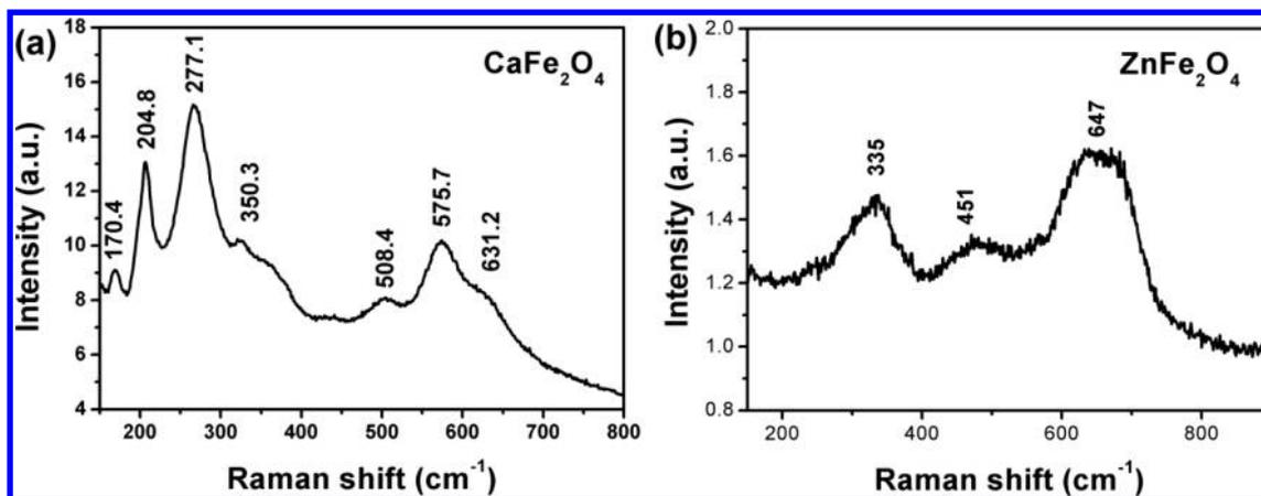
Figure 3. Raman spectra of the single-layer  $\text{CaFe}_2\text{O}_4$  and  $\text{ZnFe}_2\text{O}_4$  thin films.
