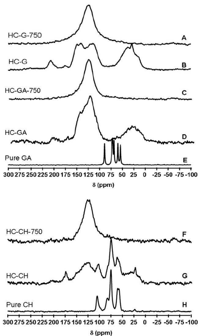
**Fig. 3 –  $^{13}\text{C}$  CP-MAS experiments performed on the pure precursors, the hydrothermally treated and carbonized (750 °C) samples.**
