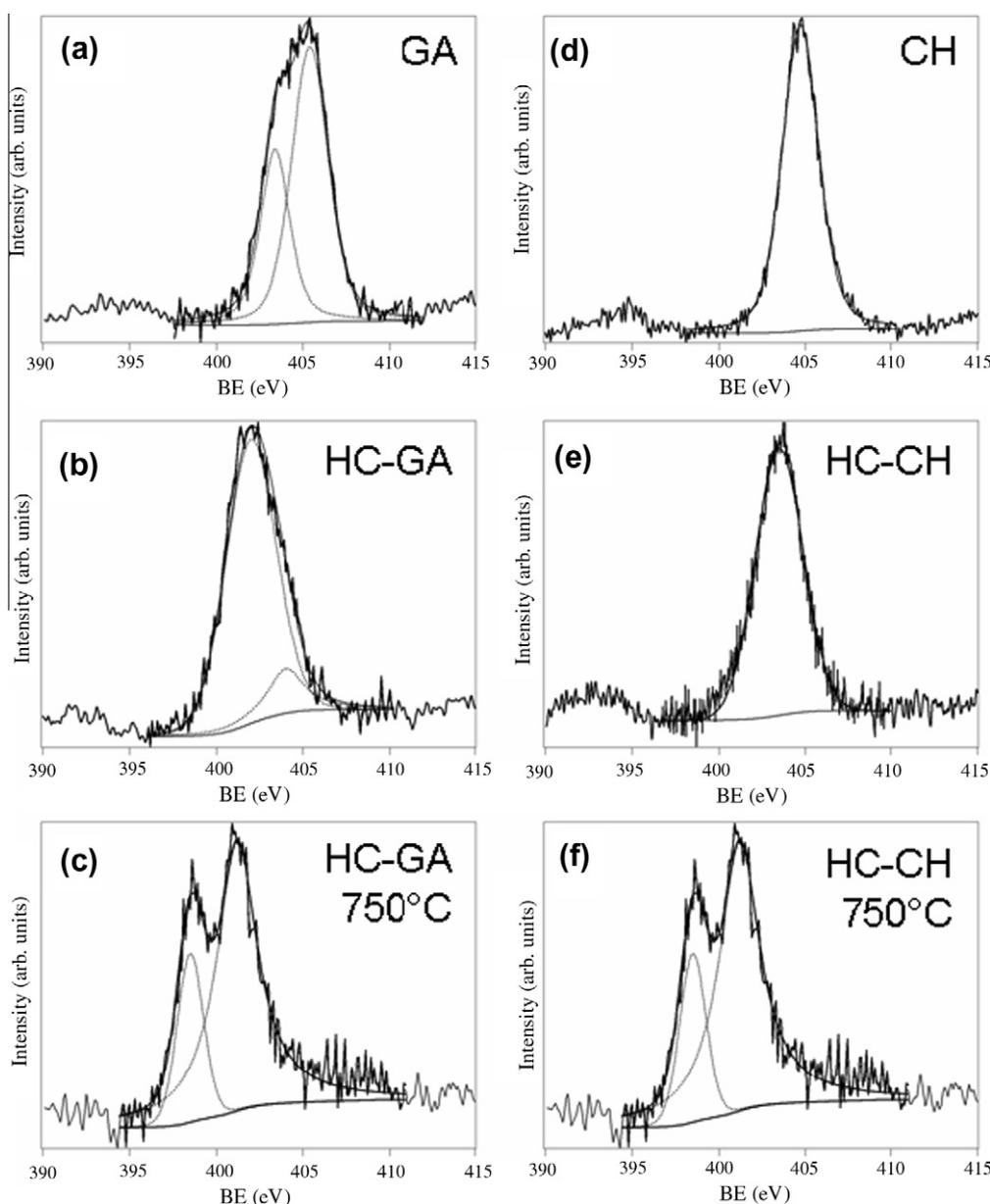
**Fig. 4** – N1s signals of the pure, hydrothermally treated and calcined glucosamine (GA) and chitosan (CH) samples. The values in the abscissa are not corrected for charging effects. Refer to discussion in the text or to Table 1 for corrected values.
