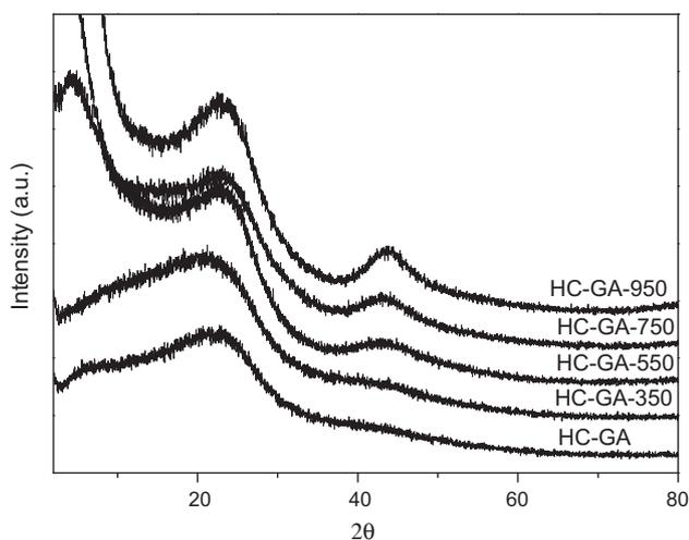
Fig. 6 – XRD profiles of the carbons obtained from glucosamine at different temperatures.
