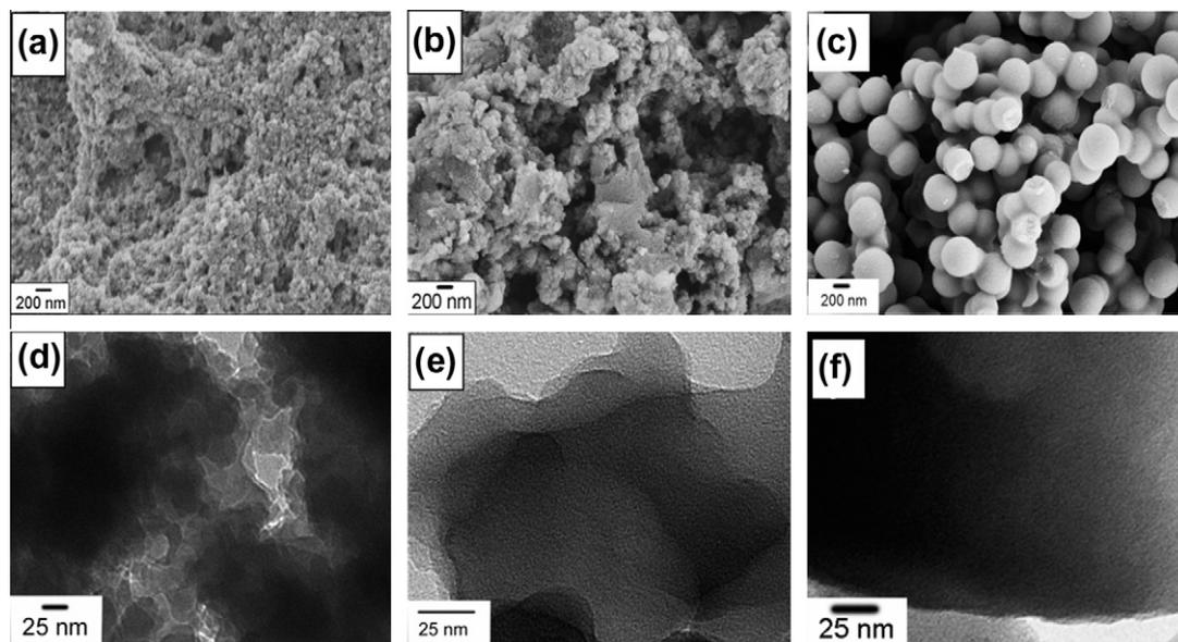
Fig. 1 – Scanning (a)–(c) and transmission (d)–(f) electron micrographs of the nitrogen-doped carbons obtained upon hydrothermal carbonization of (a) and (d) chitosan (HC-CH); (b) and (e) glucosamine (HC-GA) (c) and (f) glucose (HC-G).
