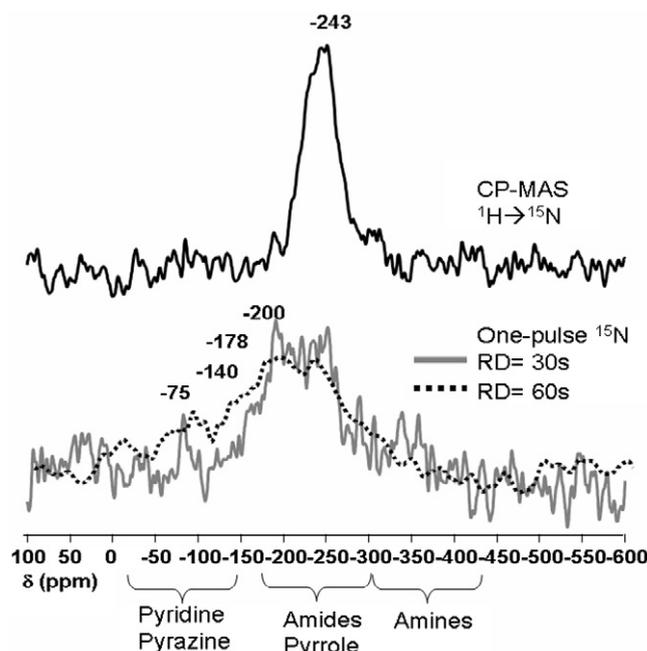
**Fig. 2 –  $^{15}\text{N}$  CP-MAS and one-pulse experiments performed on the HC-GA sample. N15 enrichment was necessary. RD = recycle delay.**
