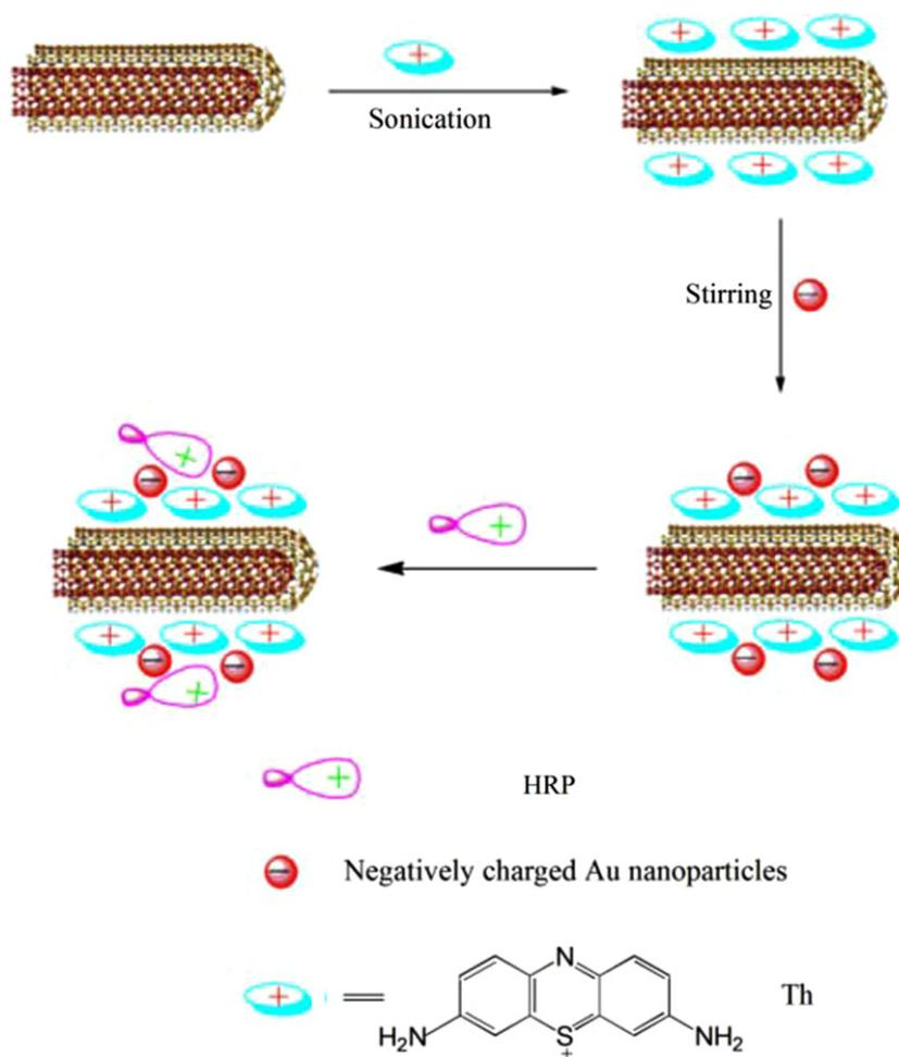
Fig. 1. Schematic illustration of the preparation procedure.
