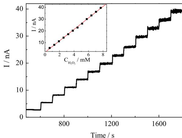
Fig. 7. Amperometric response of the HRP-MTAu composite with successive additions of  $6.4 \times 10^{-4} \text{ M H}_2\text{O}_2$  at an operating potential of 0 V.
