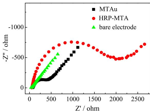
Fig. 3. Nyquist plots of bare GC electrode ( $\blacktriangle$ ), MTAu composite modified GC electrode ( $\blacksquare$ ), and HRP-MTAu film modified GC electrode ( $\bullet$ ) in 5 mM  $\text{Fe}(\text{CN})_6^{3-/4-}$  (in 1:1 ratio) in 0.1 M KCl solution, respectively. The frequency range is  $10^5$  Hz to 0.3 Hz, and the perturbation signal is 5 mV. The measurements are done at the open circuit potential.
