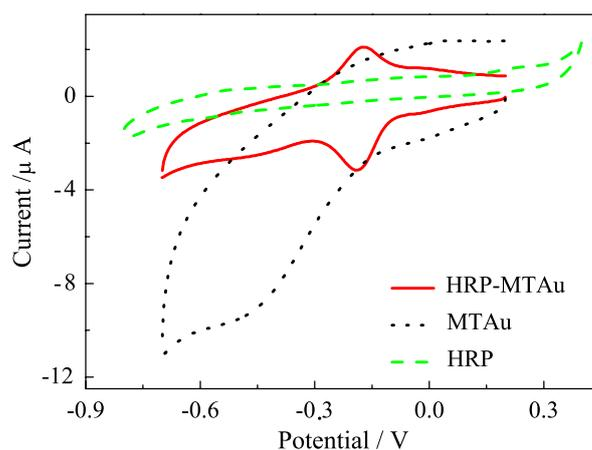
Fig. 4. Cyclic voltammograms of the HRP-MTAu film modified GC electrode (solid), MTAu composite modified GC electrode (dotted), and HRP modified GC electrode (dashed) in 0.1 M PBS (pH 7.0) saturated with  $\text{N}_2$ . Scan rate:  $0.05 \text{ V s}^{-1}$ .
