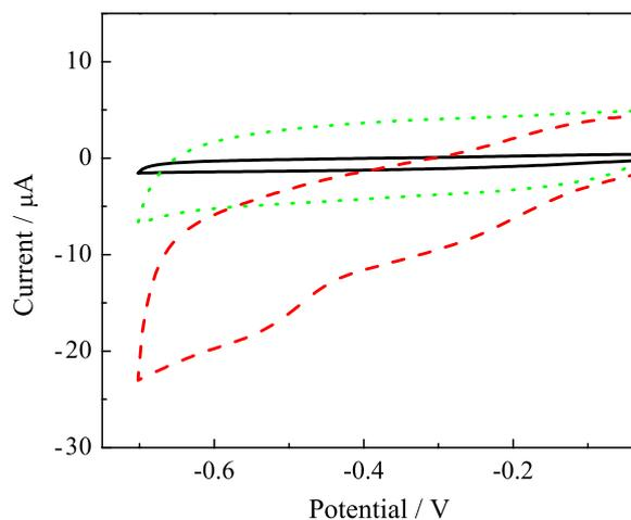
Fig. 5. Cyclic voltammograms of MWCNTs film-modified GC electrodes (dashed) and GC electrode (solid) in 0.1 M PBS (pH 7.0) with 0.5 mM  $\text{H}_2\text{O}_2$  saturated with  $\text{N}_2$  and cyclic voltammograms of MWCNTs film-modified GC electrode (dotted) in 0.1 M PBS buffer (pH 7.0) saturated with  $\text{N}_2$ . Scan rate:  $0.05 \text{ V s}^{-1}$ .
