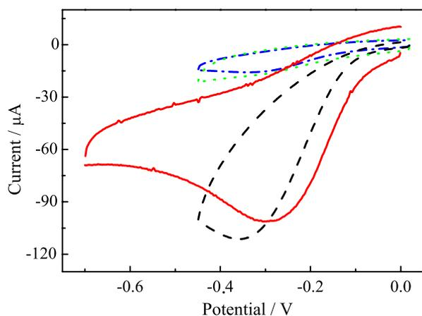
Fig. 6. Cyclic voltammograms of HRP-MTAu (solid), MTAu (dashed) film-modified GC electrodes in 0.1 M PBS (pH 7.0) with 0.5 mM  $\text{H}_2\text{O}_2$ , HRP-MTAu (dotted), MTAu (dash-dot) film-modified GC electrodes in 0.1 M PBS (pH 7.0) saturated with  $\text{N}_2$ . Scan rate:  $0.05 \text{ V s}^{-1}$ .
