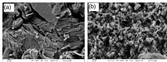
**Figure 2.** SEM images of as-prepared (a) and regenerated (b)  $g-C_3N_4$ . Scale bars are 200 nm.
