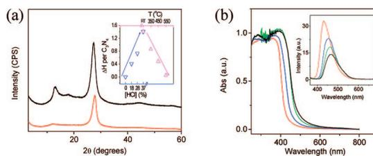
**Figure 1.** (a) XRD patterns  $g-C_3N_4$  of before (black) and after (red) the protonation with 37% HCl. Inset: Increased H number per  $C_3N_4$  unit when  $g-C_3N_4$  reacted with 18%, 28%, and 37% HCl and recovered by heating at 350, 450, and 550 °C in  $N_2$ , respectively. (b) UV–vis spectra and photoluminescence spectra (inset) of  $g-C_3N_4$  before (black) and after reaction with 18% (green), 28% (blue), and 37% HCl (red), respectively.
